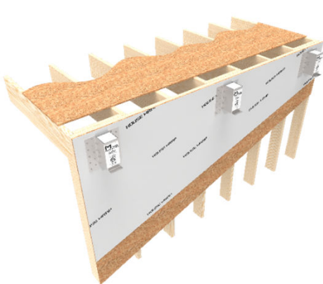
Step 1 – Mount Deck Bracket To Double Blocking
